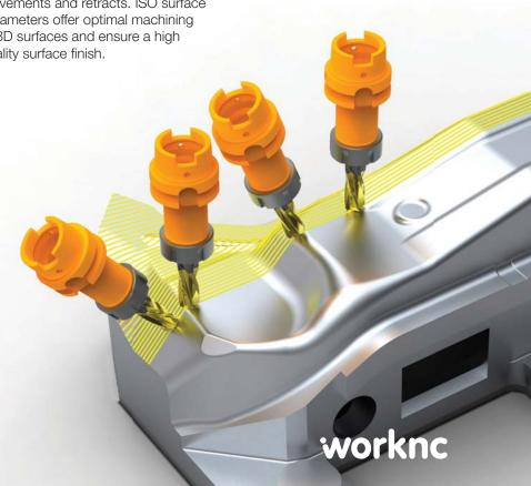
The most widely used WorkNC V22 finishing toolpaths also benefit from new features such as spiral transitions which ensure a continuous trajectory which maintains a permanent contact with the surface and offers perfect surface finish.
