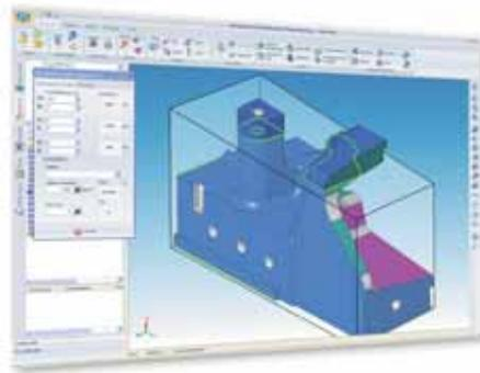
Generation of the **bounding box** of a part or a set of parts is instantaneous and provides information on the dimensions, volume and weight of the selected elements and can also be used to determine the optimal stock model required for manufacturing.
