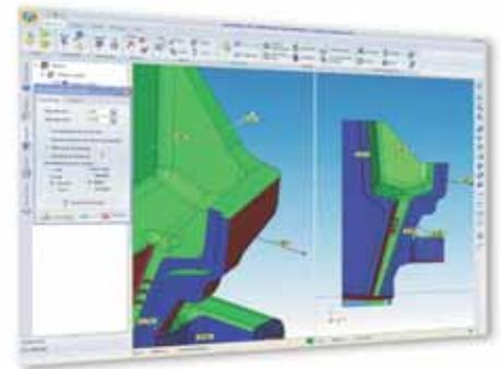
The calculation and display of **drafts and undercuts** are extremely quick, even on very big parts. WorkXPlore 3D automatically colors drafts and undercuts according to the mold stripping axis. Precise draft angle values are displayed dynamically as the mouse is dragged over the surfaces and can be inserted by default in the 3D model.
