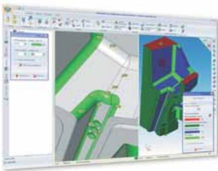
**Curvature radius and plane face analysis** is a valuable tool for users enabling fast cost and production time evaluation. The coloring of elements to be analyzed is automatic and users can insert measurement labels containing precise values of the elements selected.
