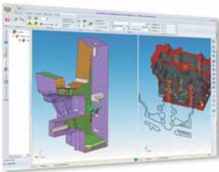
**High performance dynamic sectioning:** allows users to explore inside a part or an assembly easily and accurately. The dynamic reference controller allows users to control the section plane with the mouse in rotational and panning directions or following a guide curve. The cross section can be made visible on the 3D model or as an isolated entity and can be extracted and exported via the DXF, DWG, etc interfaces.
