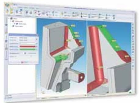
**Automatic 3D part comparison** allows real time 3D graphic display of the differences between two versions. Modifications are clearly identified by different colors to distinguish between material added and material removed.
